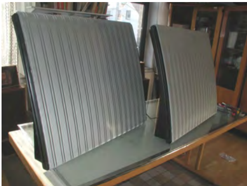
ESL57 Standard version, elastic frame for Q57 bass panel
