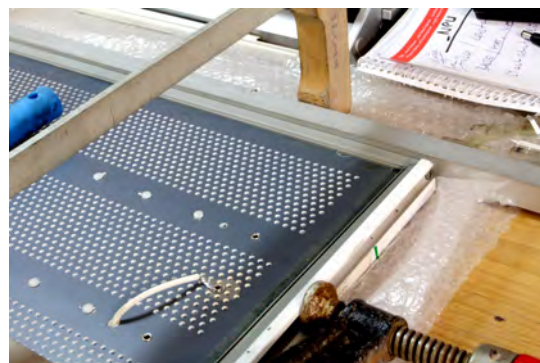
ESL57 Standard version, elastic frame for Q57 bass panel
